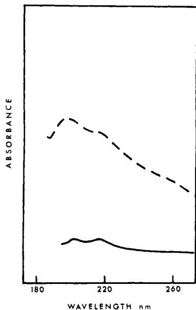
Figure 1. Ultraviolet spectra of ethyllithium vapor (—) and of the vapor–solid equilibrium mixture (---).
